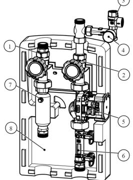
1.BALL VALVE WITH HIGH PARAMETER THERMOMETER
