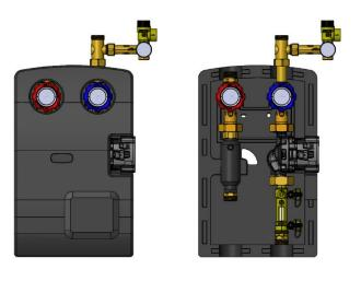
Pump group is a device that ensures and regulates the circulation of the solar fluid between the solar collectors and the tank. The group consists of a circulating pump as well as control and measuring devices. It can be used both for flat solar collectors and for vacuum collectors. The advantage of the double pump group is that it enables controlling the temperature of the solar system heating medium supply and the return.
